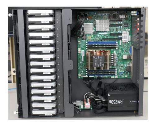
After all the drives are inserted into the slots, you can close up the unit and move on to hooking up the needed cables to your unit.
