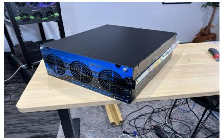
① Once the rails are attached to the side of the unit, you can install the other piece of the rail into the rack. Once again there are indicators showing which way needs to be up and which side is which.
