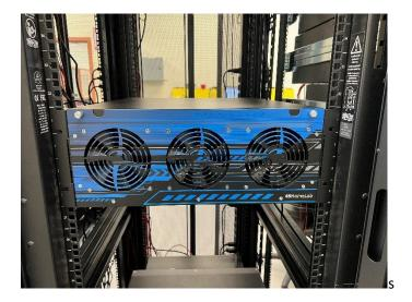
After the unit is racked the next step is to Insert the Storage Drives
