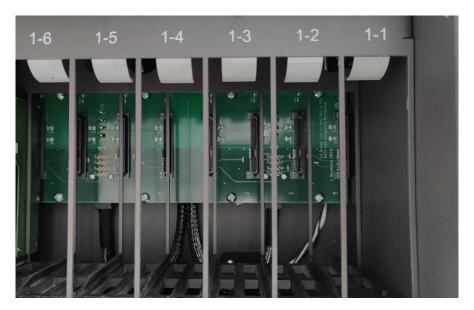
The drive should fit snugly into a slot. Make sure the back of the drive is facing the right when placing in the slot
